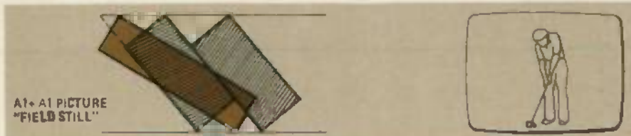
FIG. 4—USING THE DOUBLE-AZIMUTH HEAD the still-frame picture appears sharper and interference-free.
